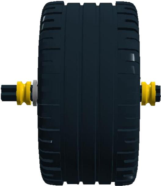
Bushings keep the wheel from sliding off the axle
