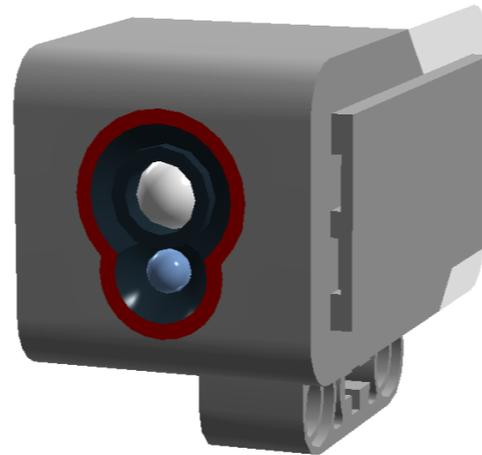
**Ambient light** - mode in which the light sensor detects the light intensity of its surroundings
