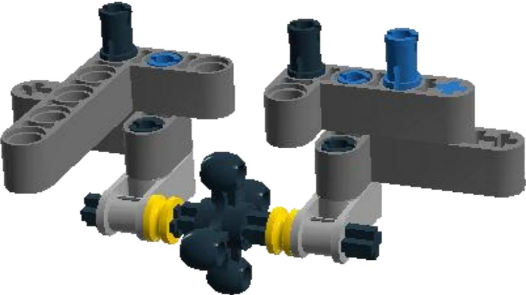
The knob wheel will slide along the ground allowing the car to turn without using a wheel
