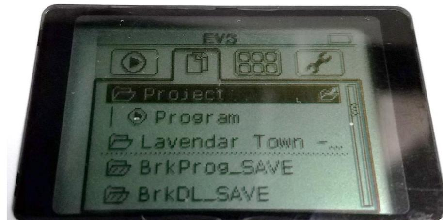
To access the files you downloaded onto the brick select the second tab then, select your project name "Project" by default, and then scroll using the arrow buttons to find your program file "Program" by default
