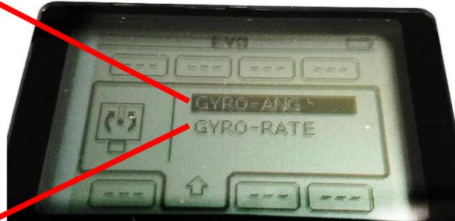
The gyro sensor displays its readings as degrees or as degrees/sec depending on selected mode (ANG or RATE)
